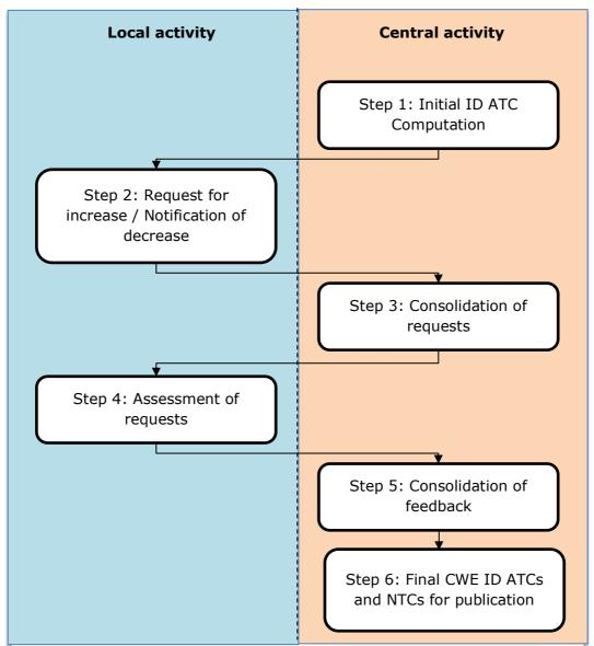
Figure 1: High-level process of ID ATC CC methodology.
