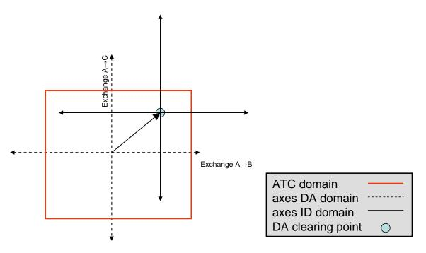
From the graphical illustration it is immediately apparent that the ATC domain remains as is, but rather the axes translate to a new origin, namely the DA clearing point.
