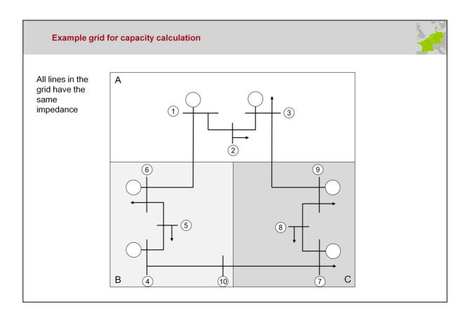
A 10-node network is used as an example to demonstrate the CWE Flow-Based (FB) capacity calculation.
